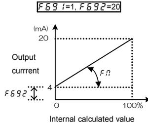
Note 1) When using the FM terminal for current output, be sure that the external load resistance is less than 750Ω.
