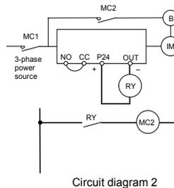
In circuit diagram 1, the brake is turned on and off through MC2 and MC3. If you do not wire it as shown in diagram 1, an over-current trip may occur because of a bound current during brake operation. (Example of running preparation ST assigned to terminal S2.)
