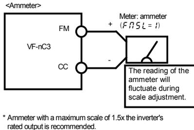
[Example of how to adjustment the FM terminal frequency meter]
