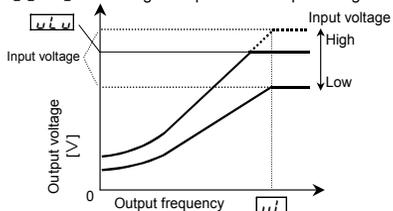
\* The above applies when V/F control mode selection parameter  $P\text{L}$  is set to "0" or "1".
