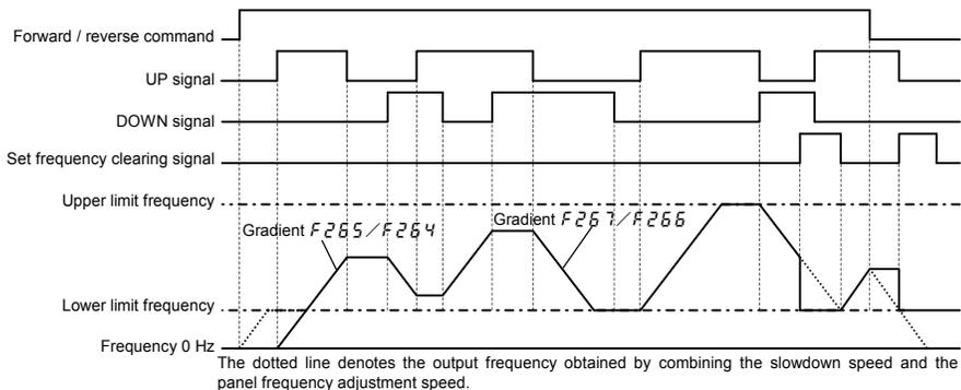
Note: If the operation frequency is set to the lower limit frequency, it will increase from 0Hz when power is turned on for the first time after the setting, and therefore the output frequency will not rise until the operation frequency reaches the lower limit frequency. (Operation at the lower limit frequency)
