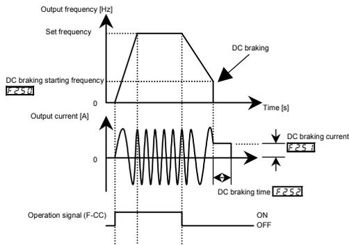
Note1: During DC braking, the overload protection sensitivity of the inverter increases. The DC braking current may be adjusted automatically to prevent tripping.
