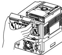
Pull the terminal cover up at an angle.
