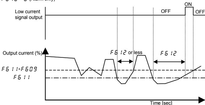
\* When setting  $F610$  to 1 (Trip), trip after low current detection time setting of  $F612$ . After tripping, the low current signal remains ON.
