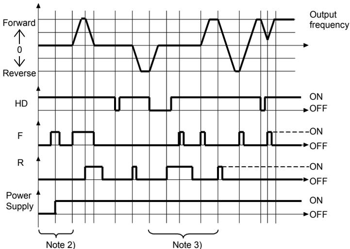
Note 1) Set  $F \setminus \setminus \setminus = \setminus$  (ST: standby) and  $\setminus \setminus \setminus \setminus = \setminus$  (terminal board) for 3 wire operation. Assign HD (operation hold) to any input terminal at input terminal selection. When assigning the S2 terminal as shown above, set  $F \setminus \setminus \setminus = \setminus$  (HD: operation hold).
