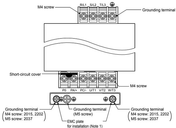
\* Bend the clips on the wiring port of the terminal cover to connect the PO, PA/+, and PC/- terminals.
