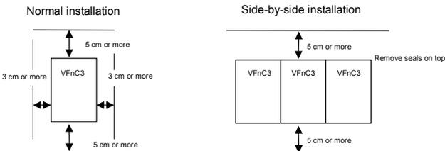
The space shown in the diagram is the minimum allowable space. Because air cooled equipment has cooling fans built in on the top or bottom surfaces, make the space on top and bottom as large as possible to allow for air passage.
