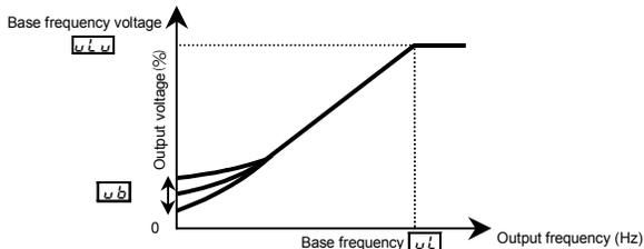
\* To increase the torque further, increase the setting value of the manual torque boost  $\omega b$ .
