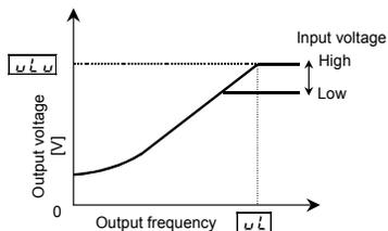
[F 30 7=2: No voltage compensation/no output voltage limit]
