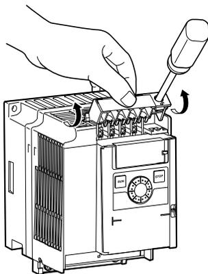
While pressing on the screwdriver, rotate the terminal cover upward to remove it.
