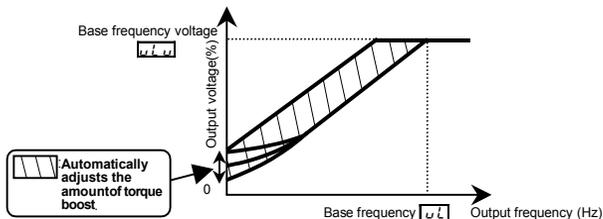
Note: This control system can oscillate and destabilize runs depending on the load. In this case, set V/F mode selection  $P_{\text{L}} = 0$  (V/F constant) and increase manual torque boost  $u_{\text{b}}$ .
