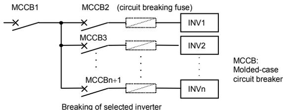
There is no fuse in the inverter's main circuit. Thus, as the diagram above shows, when more than one inverter is used on the same power line, you must select interrupting characteristics so that only MCCB2 to MCCBn+1 will trip and the MCCB1 will not trip when a short occurs in the inverter (INV1). When you cannot select the proper characteristics install a circuit interrupting fuse behind MCCB2 to MCCBn+1.
