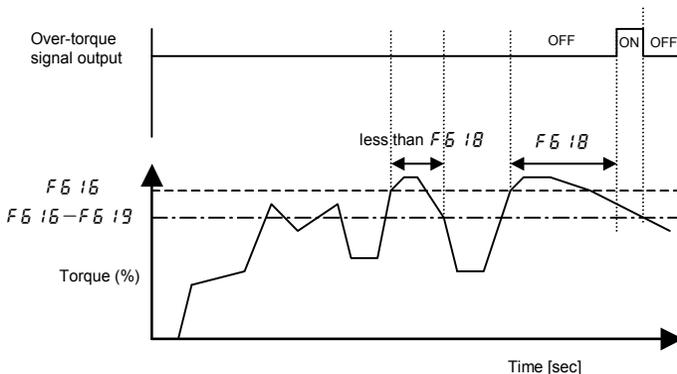
When  $F615 = 1$  (tripping), the inverter will trip if over-torque lasts for the period of time set with  $F618$ . In such a case, the over-torque signal remains ON.
