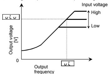
\* Note that even if the input voltage is set less than  $u_L u$ , for a base frequency of  $f_L$  or higher output frequency, then an output voltage over  $u_L u$  occurs.
