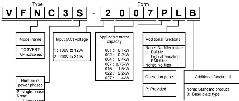
Note 1) Always shut power off first then check the ratings label of inverter held in a cabinet.
