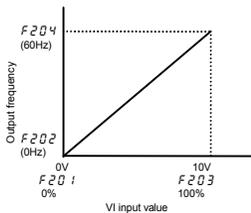
Example of 0 - 5 Vdc voltage input setting ( $F109=3$ )
