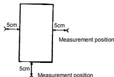
Note: The inverter is a heat-emitting body. Make sure proper space and ventilation is provided when installing in the cabinet. When installing inside a cabinet, we recommend the top seal peeled off although 40°C or less.
