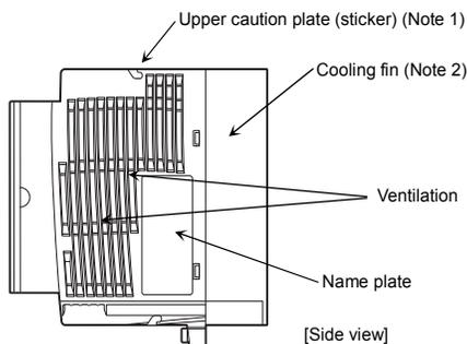
Note 1) Remove the seal as shown on the next page when installing the inverter side by side with other inverters where the ambient temperature will rise above 40°C.
