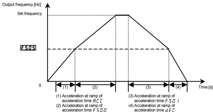
2) Switching according to terminal (switching acceleration/deceleration time by external terminal)
