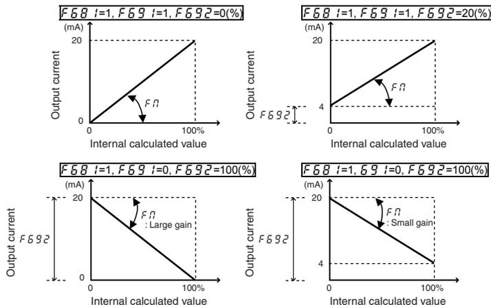
★ The analog output inclination can be adjusted using the parameter **F591**.
