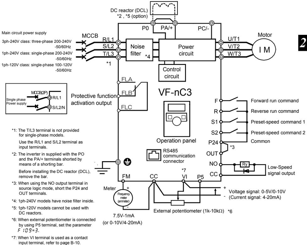
\*1: The T/L3 terminal is not provided for single-phase models.
