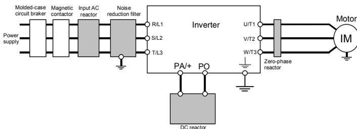
Note 1: The T/L3 terminal is not provided for any single-phase models. So if you are using single-phase models, use the R/L1 and S/L2/N terminals to connect power cables.
