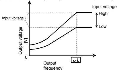
\* The above applies when V/F control mode selection parameter  $P\text{L}$  is set to "0" or "1".
