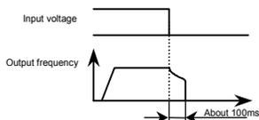
\* The time for which the operation of the motor can be continued depends on the machine inertia and load conditions. Before using this function, therefore, perform verification tests.
