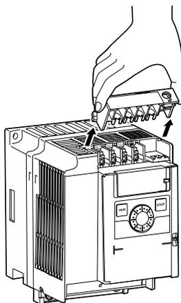
Pull the terminal cover up at an angle.
