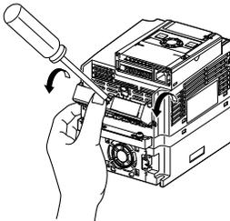
While pressing on the screwdriver, rotate the terminal cover downward to remove it.
