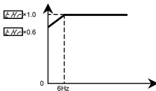
Note) The start level for motor overload reduction is fixed at 6 Hz.
