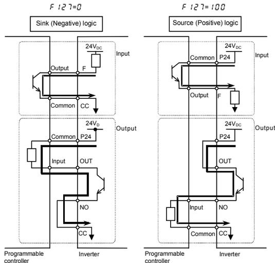
■ SINK (Negative) logic (When an external power supply is used)
