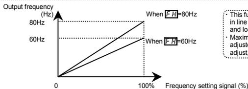
This function determines the value in line with the ratings of the motor and load.
