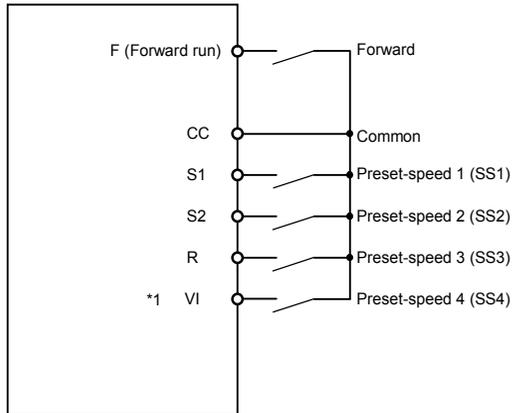
\*1: When VI terminal is used for the logic input terminal, refer to section 2.3.2 (page B-10) for details.
