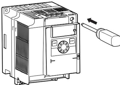
Insert a screwdriver or other thin object into the hole indicated with the □ mark.
