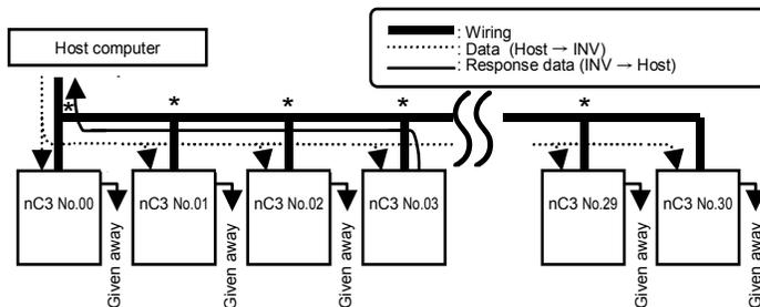
"Given away": Only the inverter with the selected inverter number conducts data processing. All other inverters, even if they have received the data, give it away and stand by to receive the next data.
