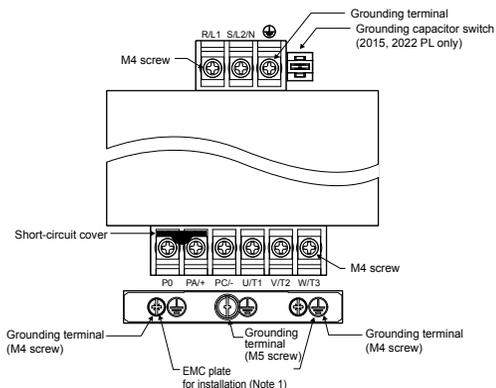
\* Bend the clips on the wiring port of the terminal cover to connect the PO, PA+, and PC/- terminals.
