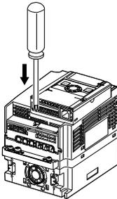
Insert a screwdriver or other thin object into the hole indicated with the ◁ mark.
