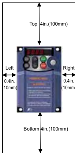
Figure 2.1 Mounting Direction and Required Clearances
