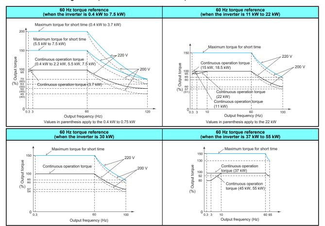
The maximum short-time torque indicates the maximum torque characteristics within 60 s.
