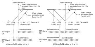
Terminal 1 (frequency setting auxiliary input) is added to the terminal 2 or 4 main speed setting signal.
