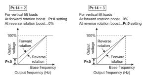
Switching applied load selection with a terminal (setting value "4, 5")
