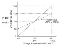
When Pr.868 (Pr.858) = "4", the terminal 1 (terminal 4) values are set to the stall prevention operation level.
