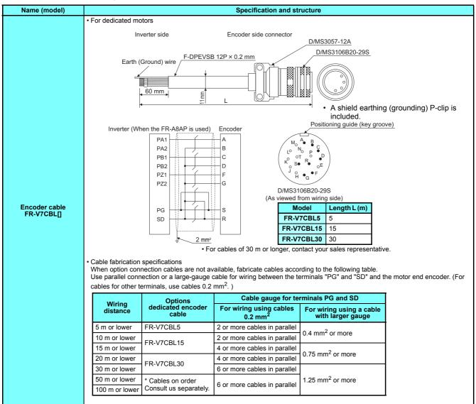
Encoder connector (DDK Ltd.) (reference) (unit: mm)
