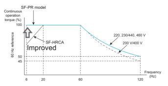
60 Hz torque reference indicates that the rated motor torque is 100% during 60 Hz operation.
