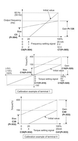
Analog input display unit changing (Pr.241) The analog input display unit (%/V/mA) for analog input bias and gain calibration can be changed.
