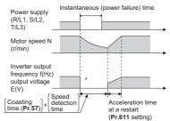
\* The output shut off timing differs according to the load condition
