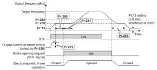
Turning ON the RT signal enables the second brake sequence function.
