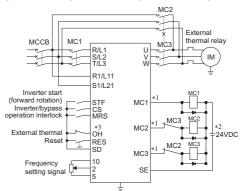
Electronic bypass sequence connection diagram (standard model)
