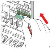
When using a single wire or a stranded wire without a blade terminal, push an open/close button all the way down with a flathead screw driver, and insert the wire.
