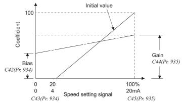
• Three methods of bias/gain adjustment for PID displayed values are the following. (a)Method to adjust any point by application of voltage (current) across the terminals 4 and 5. (b)Method to adjust any point without application of voltage (current) across terminals 4 and 5. (c)Method to adjust only the speed without adjusting the voltage (current). (For the detail of (a) to (c), *refer to page 152*.
