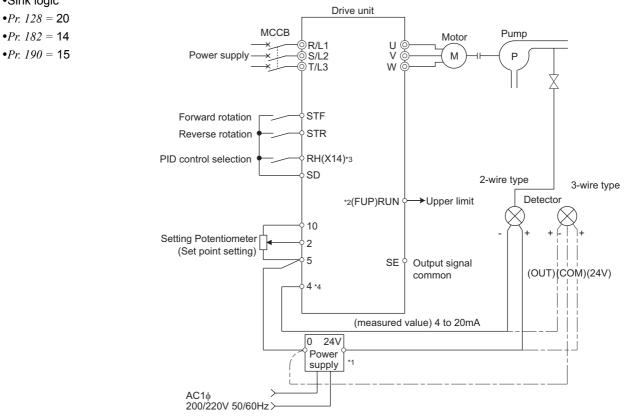
The power supply must be selected in accordance with the power specifications of the detector used. \*1
