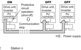
When using the RS-485 converter which receives power from the drive unit, make sure that power is provided from one drive unit only. (*Refer to the figure below.*)
