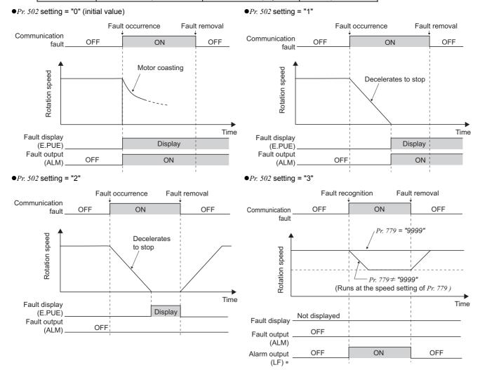
\* When a communication error is detected while Pr. 502 = "3," the alarm (LF) is output to an output terminal of the drive unit. To use the LF signal, assign the function to an output terminal by setting "98 (positive logic) or 198 (negative logic)" in Pr. 190 or Pr. 192 (Output terminal function selection).
