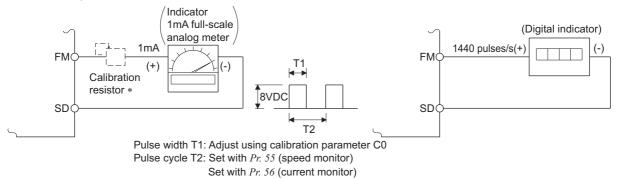
Not needed when the operation panel or parameter unit (FR-PU07) is used for calibration.
