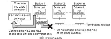
• Do not connect the PU connector to the computer's LAN board, FAX modem socket or telephone modular connector. The product could be damaged due to differences in electrical specifications.
