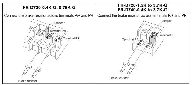
\* Do not remove the jumper across terminals P/+ and P1 except when connecting a DC reactor.
