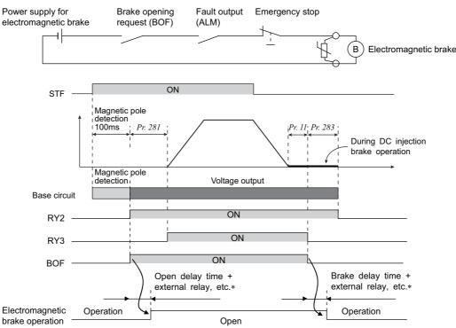
• The release of the electromagnetic brake is delayed for the electromagnetic brake release/operation time and the operation time of the relays, etc. in external circuits.
