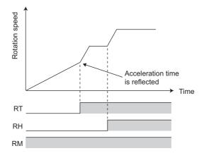
• When the RT signal is ON, the following second functions are selected at the same time.
