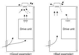
Arrangement of ventilation fan and drive unit
