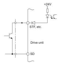
External signal input using transistor
