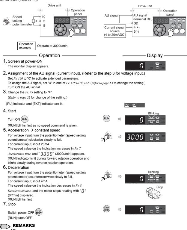
?Change the speed (3000r/min) at the maximum voltage input (5V initial value)
