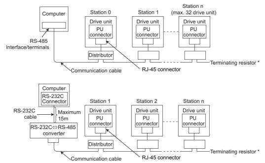
The drive units may be affected by reflection depending on the transmission speed or transmission distance. If this reflection hinders communication, provide a terminating resistor. If the PU connector is used to make a connection, use a distributor since a terminating resistor cannot be fitted. Connect the terminating resistor to only the drive unit remotest from the computer. (Terminating resistor: 100 $\Omega$ )
