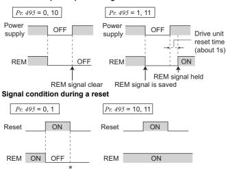
• When *Pr: 495* = "0 (initial value), 10", performing a power ON reset (including a power failure) clears the REM signal output. (The ON/OFF status of the terminals are as set in *Pr: 190* or *Pr: 192*) The *Pr: 496* setting becomes also "0".
