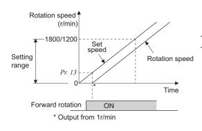
• The speed where the PM motor starts running can be set.
