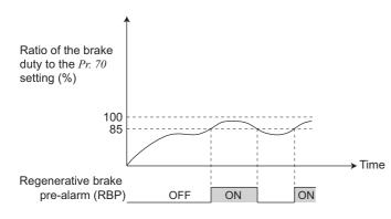
•[RB] appears on the operation panel and an alarm (RBP) signal is output when 85% of the regenerative brake duty set in *Pr*: 70 is reached. If the regenerative brake duty reaches 100% of the *Pr*: 70 setting, a regenerative overvoltage (E.OV1 to E.OV3) occurs. Note that [RB] is not displayed when *Pr*: 30 = "0".
