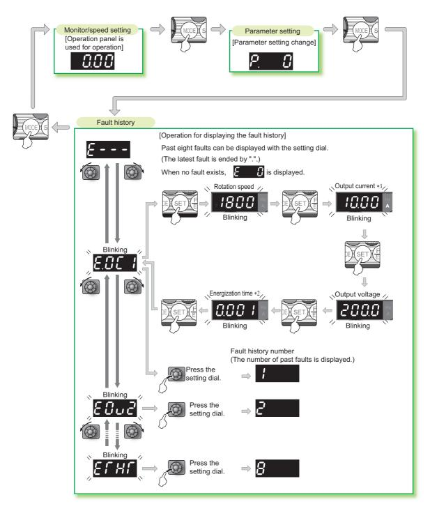
\*1 When an overcurrent trip occurs by an instantaneous overcurrent, the monitored current value saved in the fault history may be lower than the actual current that has flowed.
