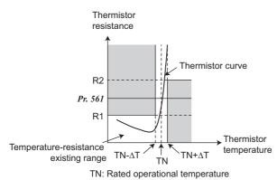
PTC thermistor output can be input to the terminals 2 and 10. When the PTC thermistor input reaches the resistance value set in *Pr. 561 PTC thermistor protection level*, drive unit outputs PTC thermistor operation error signal (E.PTC) and trips.
