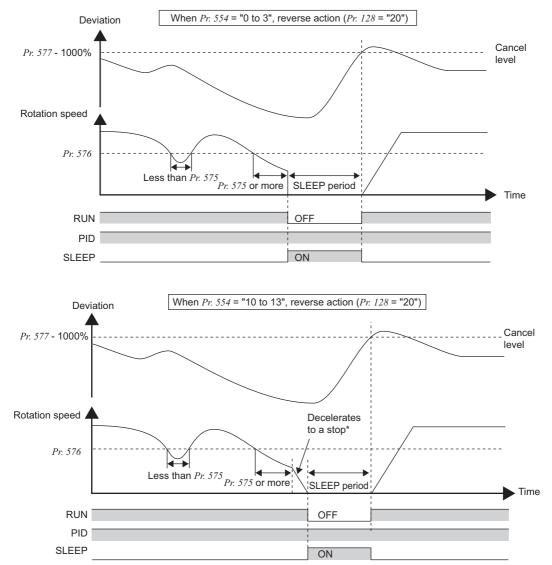
\* When the output rises to the output interruption cancel level during deceleration to a stop, output interruption gets cancelled, and the drive unit accelerates again to continue PID control. *Pr. 576 Output interruption detection level* is invalid during deceleration.
