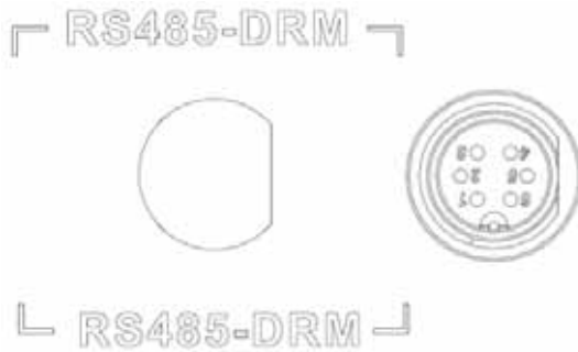
Figure 7.5 RS485-DRM pin on inverter
