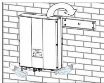
Figure 4.8 Installation of inverter
